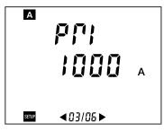
Figure 4-4 Display of the effective primary current.
