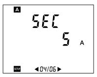
Figure 4-5 Display of the effective secondary current.
