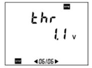
Figure 4-8 Display of the threshold voltage of the tachometer sensor.
