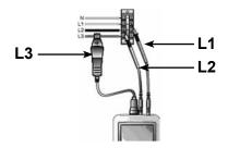
Figure 4-2 Balanced three-phase connection
