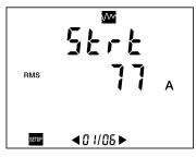
Figure 4-3 Display of start threshold current.
