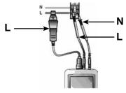
Figure 4-1 Single-phase connection
